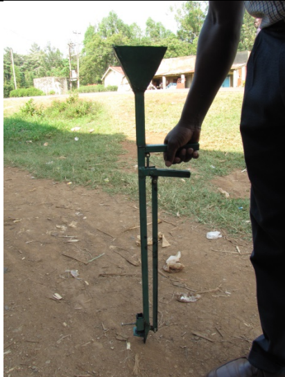
Left: a simple planter developed by a local juakali artisan in Sabatia, Kenya. Right: shallow weeders fabricated by juakali artisans in Siaya. These are in high demand because conservation agriculture is currently being promoted in western Kenya.
