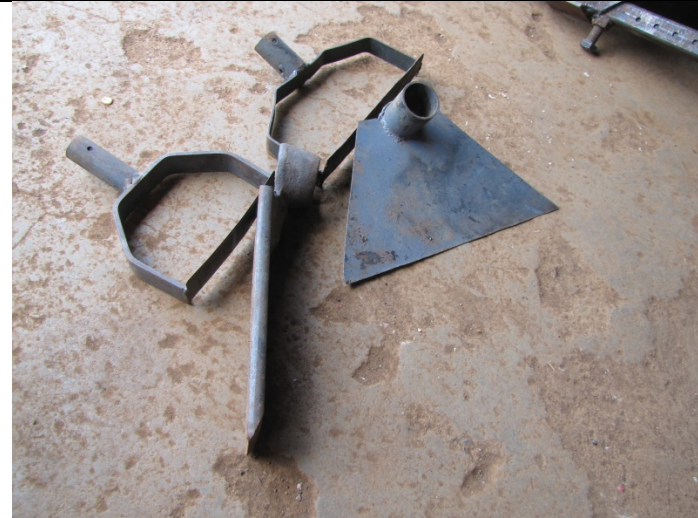
Left: a simple planter developed by a local juakali artisan in Sabatia, Kenya. Right: shallow weeders fabricated by juakali artisans in Siaya. These are in high demand because conservation agriculture is currently being promoted in western Kenya.
